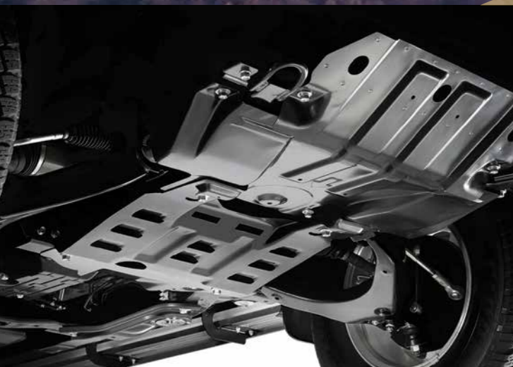
Underbody protection, front steel plate skid/shield
